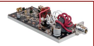
The RFP88-108-350XR is a high power, high gain Class A/AB pallet amplifier. Its XR rating ensures ruggedness for driving mismatched loads such as antennae in military or commercial communication systems. With a 0dBm input power requirement, it eliminates the need for a separate driver, making it a very cost effective solution for medium power systems applications. It is supplied on a nickel plated copper baseplate with SMA input and N output connectors.
