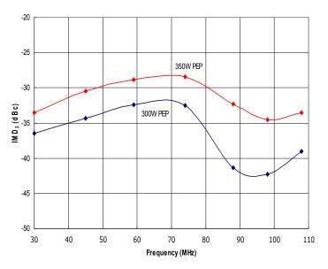
Figure 2: RFP30-108-350XR Typical IMD<sub>3</sub> @ 350W and 300W PEP,  $\Delta f$ =100kHz and  $\Delta f$ =10kHz.
