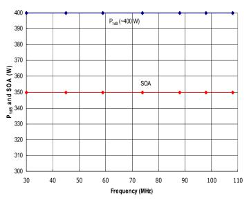
Figure 4: RFP30-108-350XR Typical  $P_{1dB}$  and Safe Operating Area (SOA). The SOA assumes a 50 ohm load and adequate cooling of output transformers. Do not exceed the SOA shown above without first contacting RFMPT to discuss your application.
