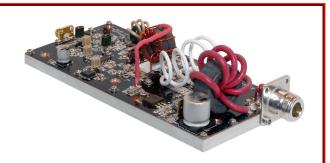
The RFP81.36-400XR is a high power, high gain Class A/AB pallet amplifier. Its XR rating ensures ruggedness for driving mismatched loads in demanding 81.36MHz ISM applications. With a OdBm input power requirement, it eliminates the need for a separate driver, making it a very cost effective solution for medium power systems applications. It is supplied on a nickel plated copper baseplate with SMA input and N output connectors.
