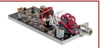
The RFP40.68-400XR is a high power, high gain Class A/AB pallet amplifier. Its XR rating ensures ruggedness for driving mismatched loads in demanding 40.68MHz ISM applications. With a 0dBm input power requirement, it eliminates the need for a separate driver, making it a very cost effective solution for medium power systems applications. It is supplied on a nickel plated copper baseplate with SMA input and N output connectors.
