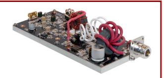
The RFP27.12-400XR is a high power, high gain Class A/AB pallet amplifier. Its XR rating ensures ruggedness for driving mismatched loads in demanding 27.12MHz ISM applications. With a 0dBm input power requirement, it eliminates the need for a separate driver, making it a very cost effective solution for medium power systems applications. It is supplied on a nickel plated copper baseplate with SMA input and N output connectors.
