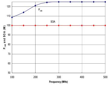
Figure 4: RFM100-500-100-HSD Typical  $P_{1dB}$  and Safe Operating Area (SOA). Do not exceed the SOA shown above without first contacting RFMPT to discuss your application.
