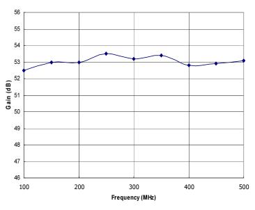
Figure 1: RFM100-500-100-HSD Typical Gain @ Pout=100W.
