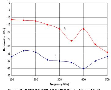
Figure 3: RFM100-500-100-HSD Typical  $f_2$  and  $f_3$  @  $P_{out}$ =100W.
