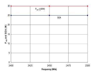
Figure 3: MWM2400-2500-25 Typical P<sub>1dB</sub> and Safe Operating Area (SOA). Do not exceed the SOA shown above without first contacting RFMPT to discuss your application.
